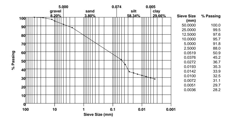
Due to the percentages of granular on cohesive material, this soil is classified as a sandy clay. Based on these results and the Safety Codes Council & Alberta Private Sewage Systems Standard of Practices (1999), the soil is not suitable for disposal fields without further testing.
