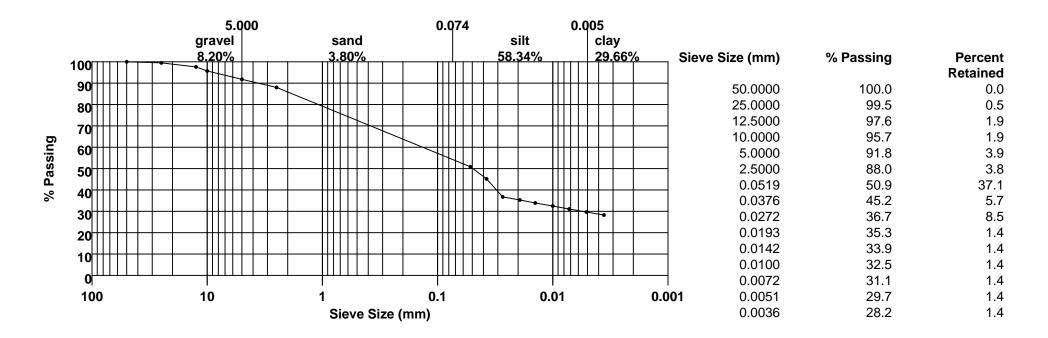
Due to the percentages of granular on cohesive material, this soil is classified as a sandy clay. Based on these results and the Safety Codes Council & Alberta Private Sewage Systems Standard of Practices (1999), the soil is not suitable for disposal fields without further testing.
