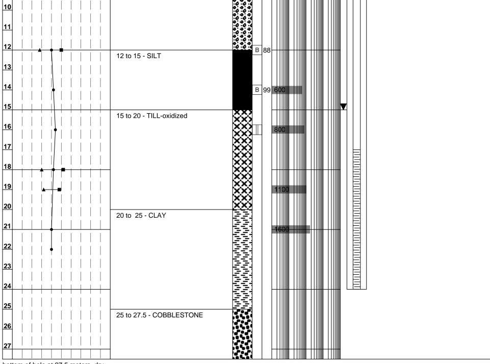
bottom of hole at 27.5 meters, dry at completion, standpipe installed
